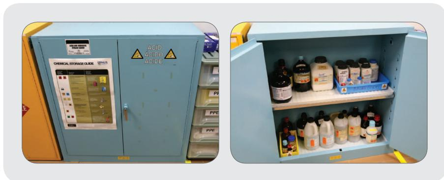
Figure 12: Storage cabinet for corrosive chemicals with cabinet doors closed (left) and open (right).
