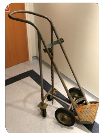
Figure 18: A cylinder cart specially designed for moving gas cylinders.
